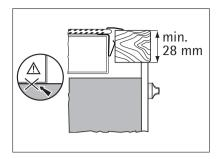
If you use a protection box (the additional accesi sory<sup>1)</sup>), the protective floor directly below the appliance is not necessary.
