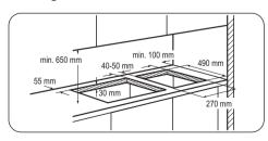
If several 30 cm hobs are to be installed side by side into the same cut out, an assembly kit including a support side bracket and supplementary seals is available at our Service Centres.
