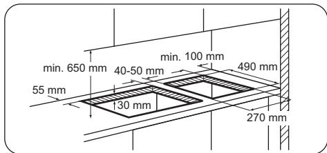
If several 30 cm hobs are to be installed side by side into the same cut out, an assembly kit including a support side bracket and supplementary seals is available at our Authorised Service Centres. The relevant installation instructions are supplied within the kit package.
