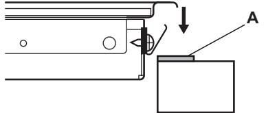
Place the sealing gasket A all around the edge of the cut out.
