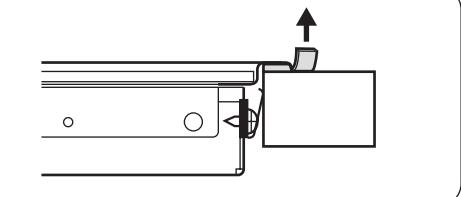
Fit the hob in the cut out and push it down until comes in contact with the kitchen top surface. then remove the excess sealing.
