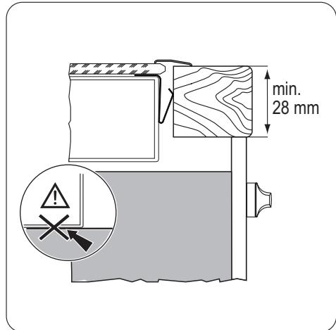
**i** If you use a protection box (the additional accessory<sup>1)</sup>), the protective floor directly below the appliance is not necessary.
