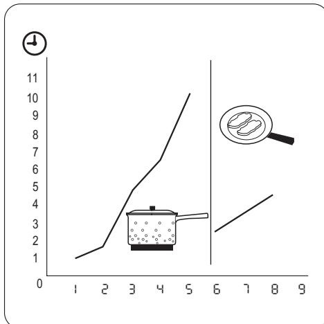
You can get a necessary heat setting in a shorter time if you activate the Automatic Heat Up function. This function sets the highest heat setting for some time (see the illustration), and then decreases to the necessary heat setting. To start the Automatic Heat Up function the cooking zone must be cold (no
